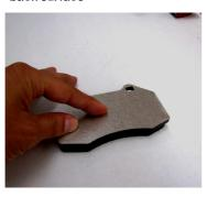
Apply the P-DEF plate and maintain a light pressure for few seconds until the glue sets.
