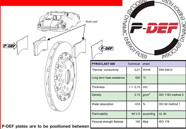
the brake lining and the calliper's pistons, creating a <u>barrier for the passage of the heat</u> given off during the braking.
