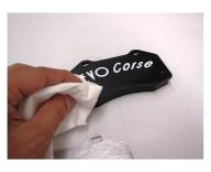
Clean up carefully the brake pad back surface
