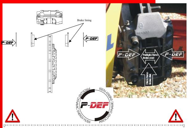
After cleaning, it is recommended to glue the plate with a few drops of adhesive on the brake lining's back. This insures making it a one piece lining to avoid any possible problems with racing rules.
